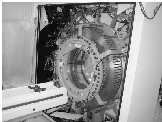
Figure 1. Photograph of the inside of a PET scanner. It consists of a ring-shaped gantry with many scintillation crystals.
