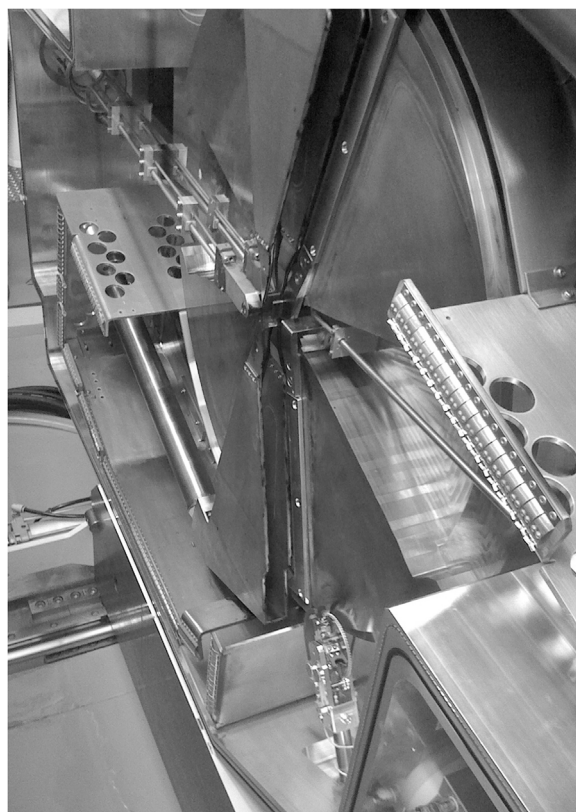
Figure 2. Photograph of the inside of a cyclotron. The cyclotron generates a proton or deuteron beam, which collides with the appropriate target (for example, water with enriched ^{18}\text{O} to generate ^{18}\text{F} ).
