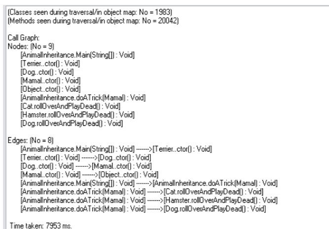
Figure 4. Execution of call graph analyzer with class hierarchy analysis
