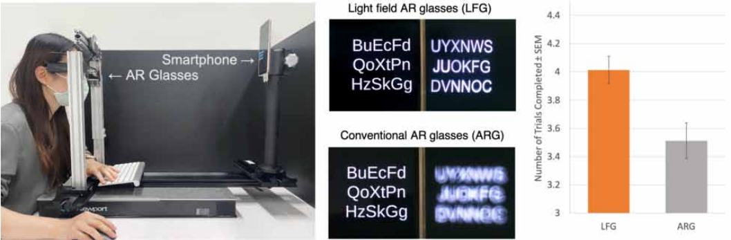
Figure 1. We present a series of text-based visual search tasks to systematically and quantitatively test human visual performance under the influence of vergence-accommodation conflict (VAC). From left to right: experimental setup, example visual content, and experimental results. Each visual content example includes two side-by-side text blocks. The left text block is displayed by a smartphone, and the right text block by a pair of AR glasses.
