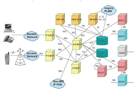
Figure 1. The architecture of the 3GPP IP multimedia subsystem (IMS)
