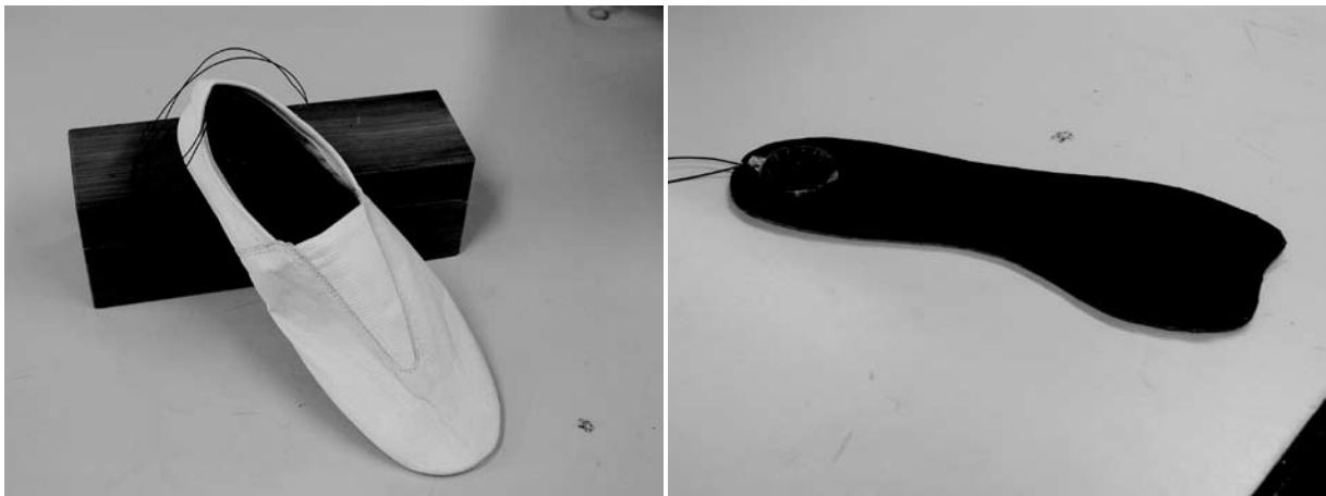
Figure 1. Sensorized shoe for marking the gait cycle
