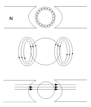
Figure 1 (c) shows the main magnetic field due to field magnets. This field is obviously horizontal. So, we see both armature and the main fields (individually) are at right angel to each other. The armature field is also called as cross field.
