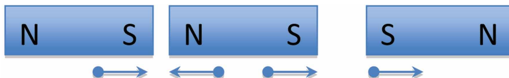
Figure 1. Behavior of magnets (attraction and repulsion factors)
