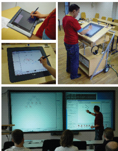
Figure 1. Pen-based interfaces commonly used in classrooms: Tablet PC (top left), graphics tablets (middle left and top right), and electronic whiteboards (bottom)
