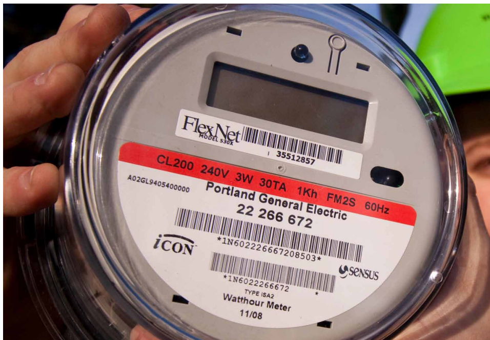
Figure 1. Residential smart meter
