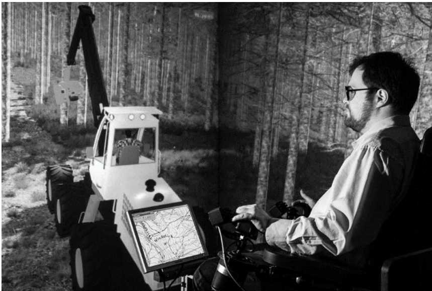
Figure 1. Driver training by means of an advanced forest machine simulator
