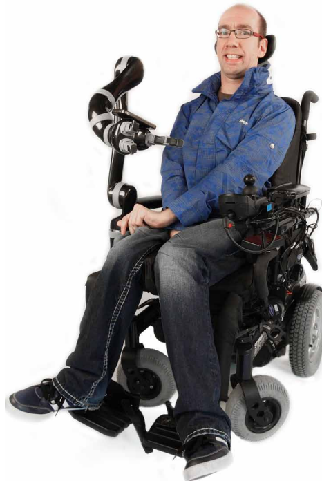
Figure 1. JACO mounted on a powered wheelchair. Figure courtesy of Kinova.
