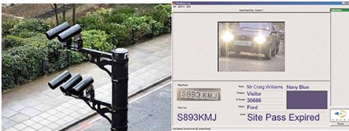
Figure 1. An example of a fixed ANPR camera and an associated read (Lyddon, 2016) (SAE Systems, 2022).
