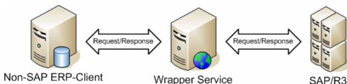
Figure 1. Communication between non-SAP systems and SAP/R3 Systems on the basis of Web Services
