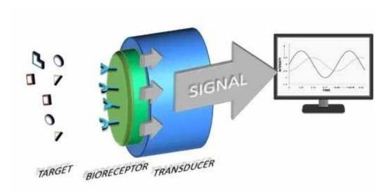
Figure 1. Biosensor structure and transducing mechanism
